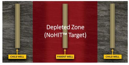
Parent well preload treatment with NoHIT™ protects the parent and encourages child fracs to move into undepleted high pressure intervals
